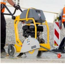
The largest water tank in its class: 20 I on the BFS735 and 940 or 32 I on the BFS1345 and 1350.
