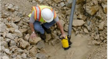
Electric submersible pumps that are safe to dry run: even during long intermittent operation due to lack of water thanks to the built-in oil lifter.
