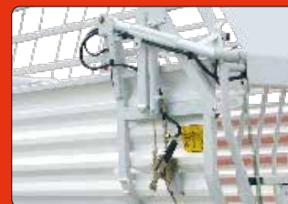
Optionally with hydraulic door opener , for convenient opening of the door from the driver's seat.
