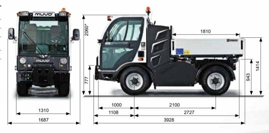
Dimensions are shown in mm. \*Depends on mounted attachment/s.
