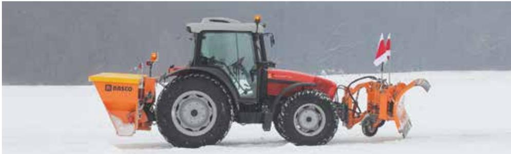
The spreader is mounted on the standard rear leverage of the tractor. The spreader is powered by the tractor's hydraulic system, and only one pair of hydraulic couplings is needed.
