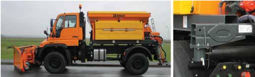
Fast and simple mounting using the existing sub-chassis of the vehicle tipper box and a special carrying frame on the spreader. The simplest mounting method that enables complete vehicle multifunctionality.
