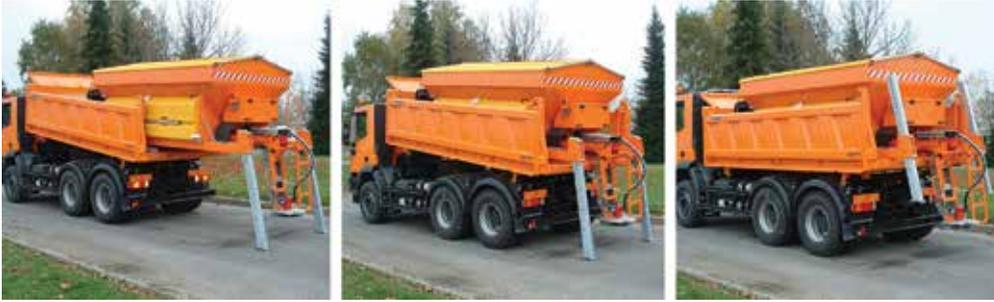
System for mounting the spreader in a tipper box using RO-RO (Roll-On, Roll-Off) legs and rollers on the device itself is the most common and simplest mounting method. The spreader is easily attached to the tipper box by using tension chains or belts.
