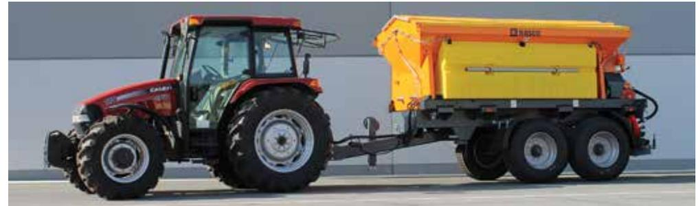
Spreaders are mounted on tractor or truck trailers, thus becoming independent from the towing vehicle.
