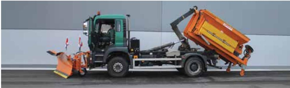
A specially adjusted spreader frame enables simple mounting on vehicles equipped with a system for raising devices using a hook.
