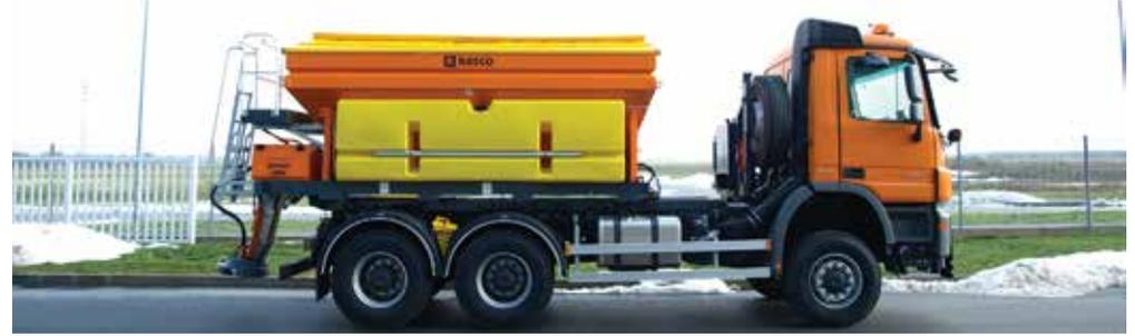
Suitable in situations when the vehicle is used exclusively for road maintenance. Different devices, including the spreader, can be easily replaced on the vehicle chassis using specially designed carrying frames.
