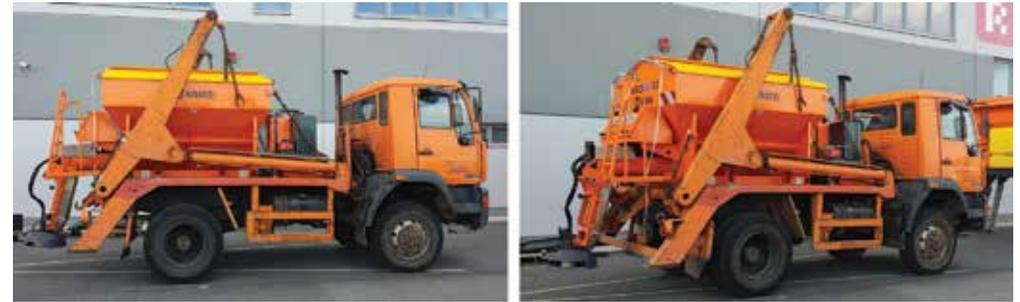
Simple mounting on vehicles equipped with a container lifting system is enabled by special attachment points on the sides of the spreader.
