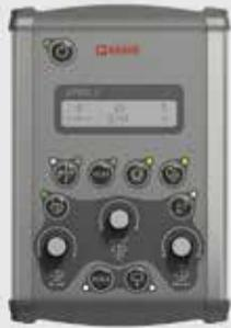
This control unit is intended for the control of smaller spreaders used on more demanding road sections. Based on more complex EPOS units, but lacks the system of feedback connections. However, its operating precision is still very high. Ergonomic and transparent, with an intuitive distribution of controls for managing the operation of spreader functions and a two-row LCD screen showing the currently set spreading parameters.
