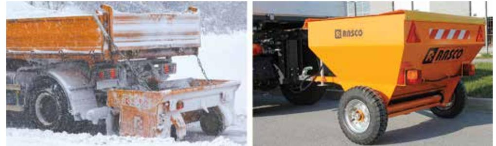
Mounting is performed by a rear hook or attaching the vehicle to the drawbar. The spreader is secured from side movements during reverse driving with chains attached to the vehicle box.
