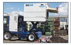
Very large volumes of dry collected waste. 6 m³ hopper and 6000 kg payload is the highest capacity on the market, allowing long working shifts.
